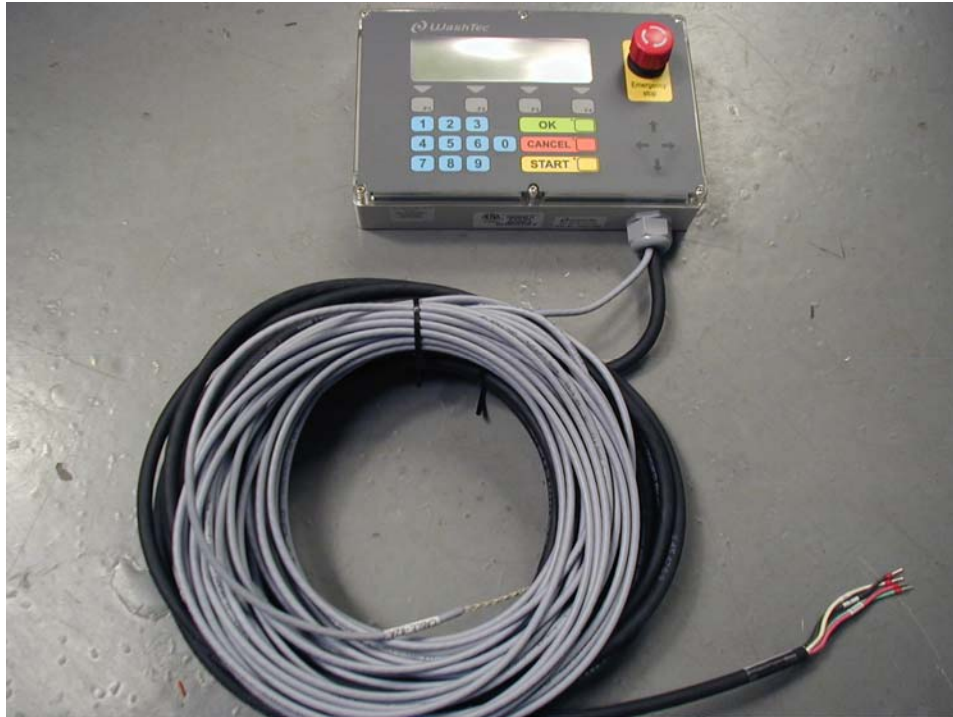
Figure 3.05-04, CP0 with CAN Communication cable, and E-Stop cable
