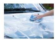
Hand washing **can leave scratches** on a vehicle's finish as a result of using porous sponges that hold on to small pieces of grit and dirt. The same goes for drying with old towels
