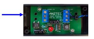
Connect 24VAC wash start signal lines from your car wash into connections 1 and 3 on connector S1 in the Wash Open Interface Unit
